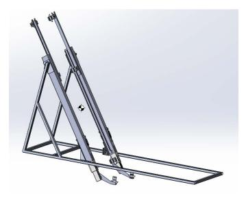
Figure 2.10: Frame for vertical conveyor.
