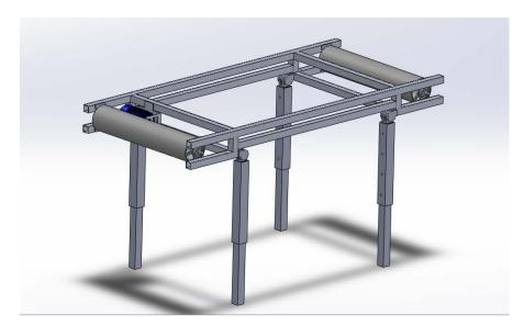
Figure 3.2: Modular conveyor sections with legs extended
