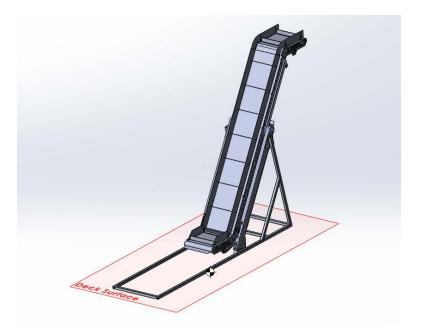
Figure 2.13: Fully assembled and raised vertical conveyor system
